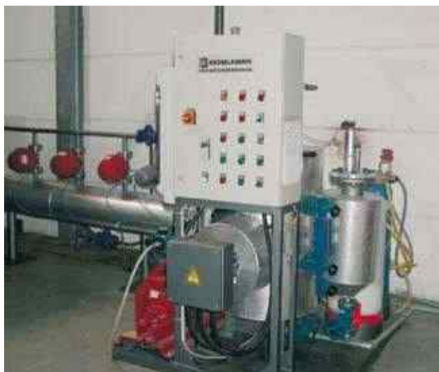
Test stand sterilization process simulation. Cycle and lifetime testing of diaphragms and valves with saturated steam
