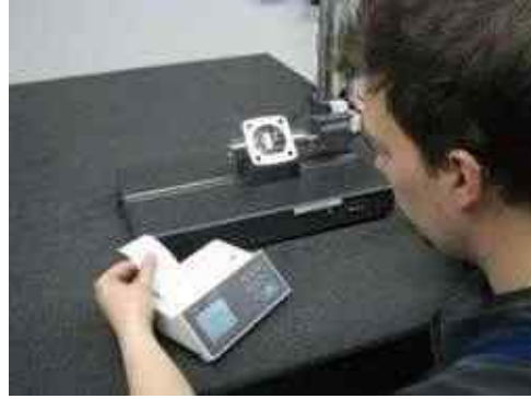
The surface finish, roughness, is measured and recorded at defined reference points according to DIN EN ISO 4287.
