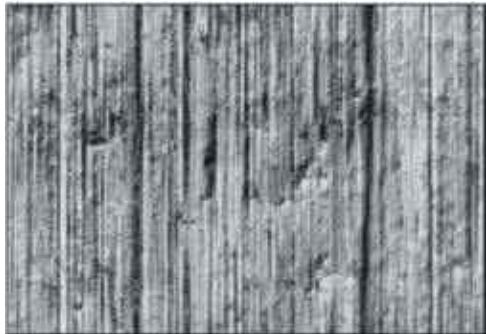
Microscopic view of mechanically polished surface with grit 400 \text{Ra } 0,25 \mu\text{m} / 10 \mu\text{-inch}
