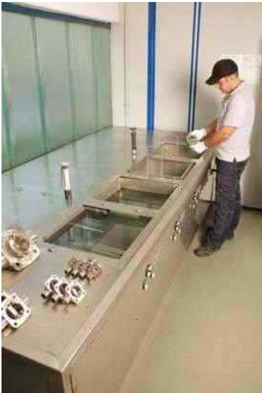
Ultrasonic cleaning of valve bodies
