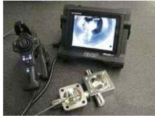
Borescope inspection of the interior surface and weld seams of valves for aseptic applications
