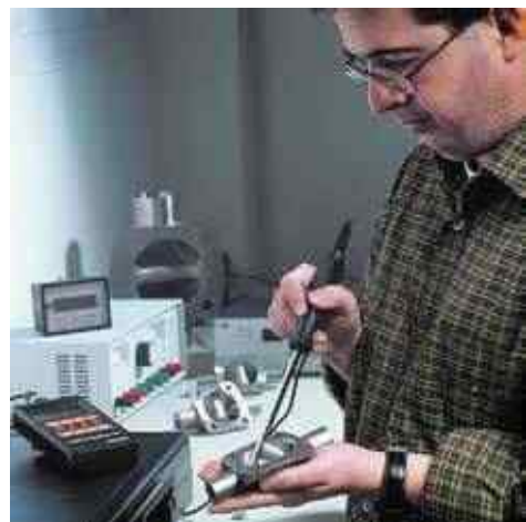
Delta Ferrite measurement of stainless steel valve bodies
